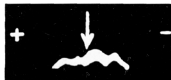
Fig. 2.—Descending boundary pattern of pooled Buthus judaicus venom analysed in Perkin-Elmer electrophoresis apparatus at total protein concentration of about 1\% , barbital buffer pH 8.6 , ionic strength 0.1 and 1^{\circ}\text{C} . The venom was dialyzed for 24 h prior to analysis. The mobilities of the five fractions from left to right, are in \text{cm}^2 \cdot \text{V}^{-1} \cdot \text{s}^{-1} \times 10^{-5} : A_1 : -3.36 , A_2 : -1.57 , K_3 : +0.58 , K_2 : +1.9 and K_1 : +2.2 . The arrow indicates the position of the boundary at start. The non-moving O fraction encountered in paper electropherogram was not discernible in the moving boundary pattern. The distended peaks of the cathodic fractions indicate their heterogeneity.
